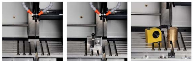
Large cutting chamber with various clamping devices
