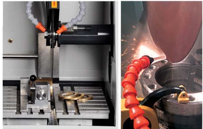
Multi-slice automatic serial cutting of plane parallel sections
